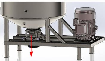
2) When service is required, the seal/bearing cartridge is lowered onto a carriage with rollers that rest on the mixer frame.
