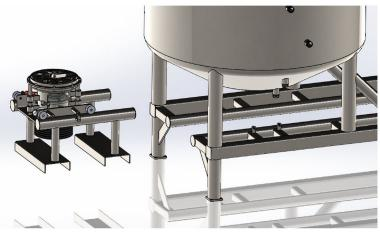
4) The seal/bearing cartidge and carriage can then be secured to a pallet jack trolley and then removed to a service area where all the mixer internals can be serviced.
