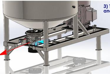
3) The carriage is then disengaged from the frame and can be rolled onto the mixer frame.
